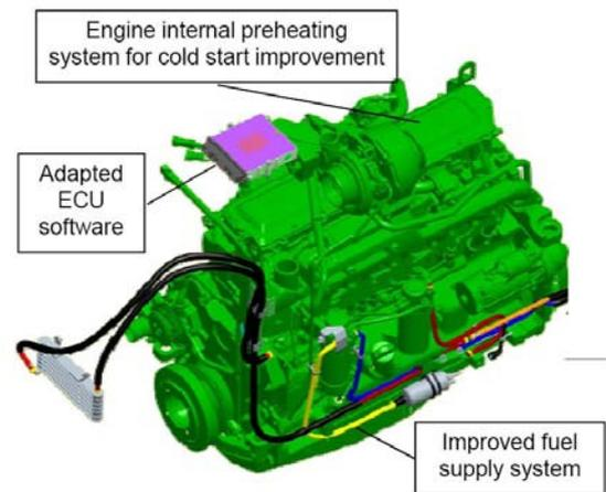
**Figure 2:** The VWP-JD advanced engine concept.
