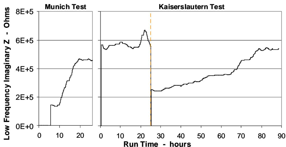
The plot shows the filtered Low Frequency imaginary impedance for both tests. At worst the peak was only just reached for the two drain intervals; hence, the surface protection functionality of the lubricant remained good during both intervals. Assuming the same lubricant
