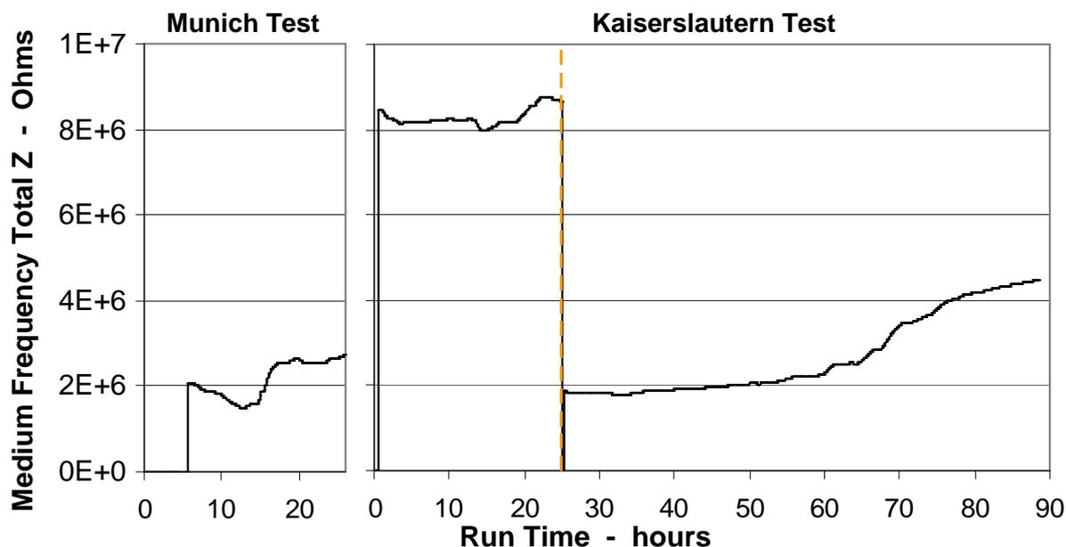
The plot shows the filtered Medium Frequency total impedance for both tests. Since the peak was not reached for the one drain interval of the Munich test or for either drain interval Kaiserslautern test, the contaminant control functionality of the lubricants remained very good throughout both tests.
