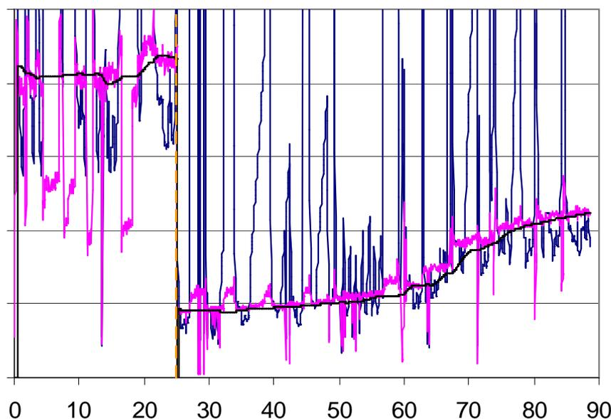
The MFI sensor outputs high, medium and low frequency (HF, MF and LF respectively) impedances and temperature every ~3 minutes. The raw outputs were logged and an off-line MFI algorithm uses the temperature data to normalize/compensate the raw data to a single temperature and then filters for temperature range and rate and for noise. The algorithm compares the filtered data trends to thresholds to determine lubricant condition and to identify when oil changes are needed.
