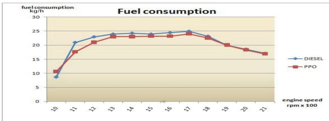
Figure 4. Fuel consumption for different engine's load
