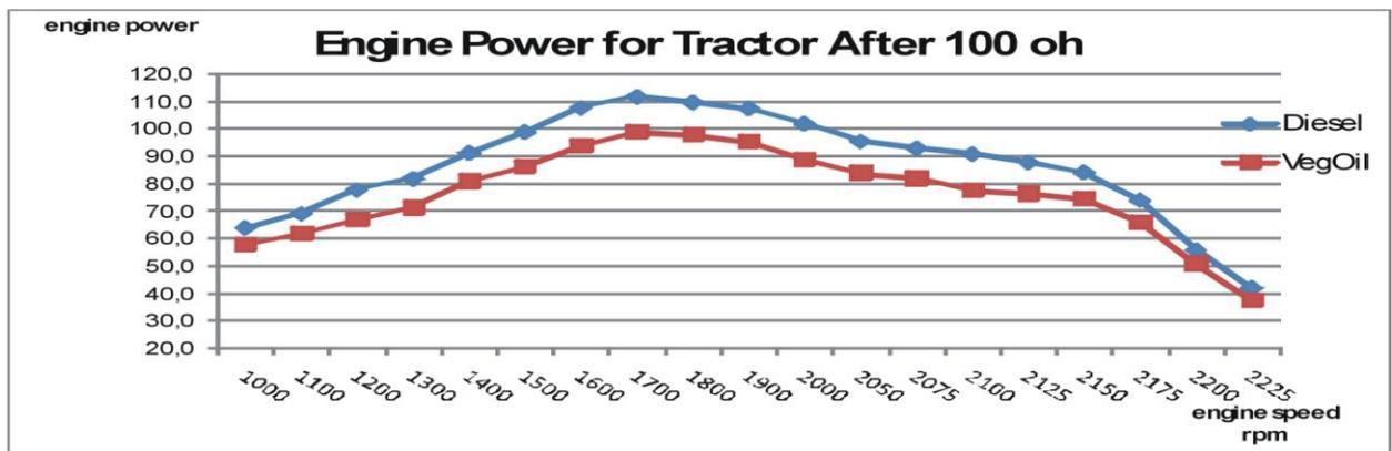
Figure 3. Engine Power for tractor run on diesel or on vegoil
