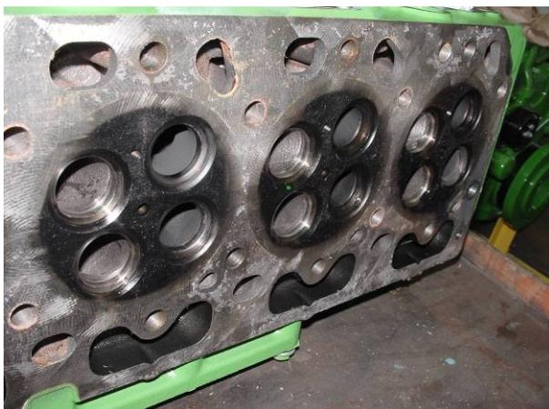
Fig. 5: part of the cylinder head (from the bottom)
