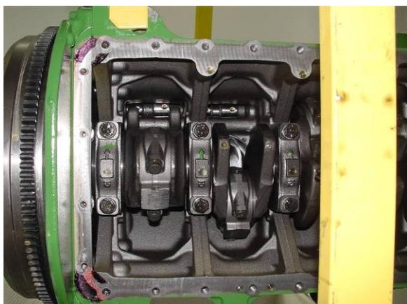
Fig. 3: Snapshot from the bottom after disassembling of the cylinder 1 oil pan (cylinder 6 next to the flywheel)
