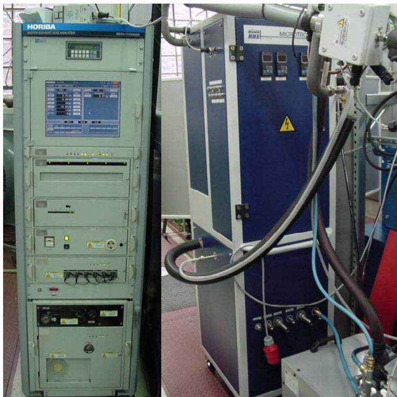
*Fig. 9: Exhaust measurement (left: Horiba Mexa, right: Nova Microtrol)*
