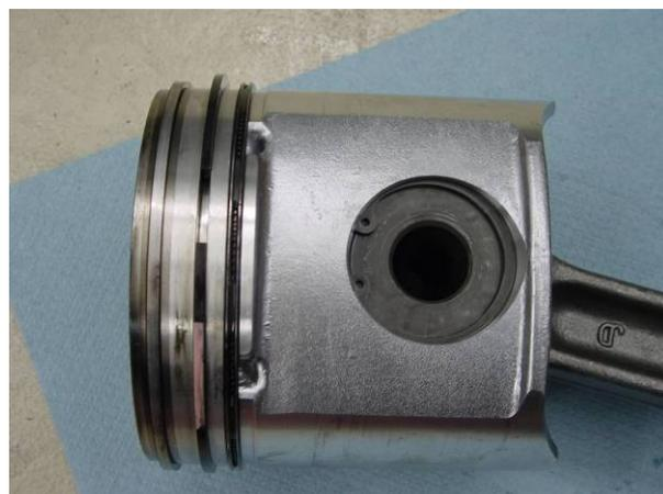
Fig. 6: piston with piston rings
