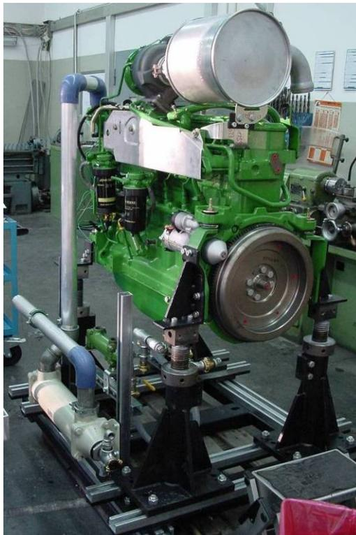
*Fig. 7: Engine on framework, cooling system assembly*
