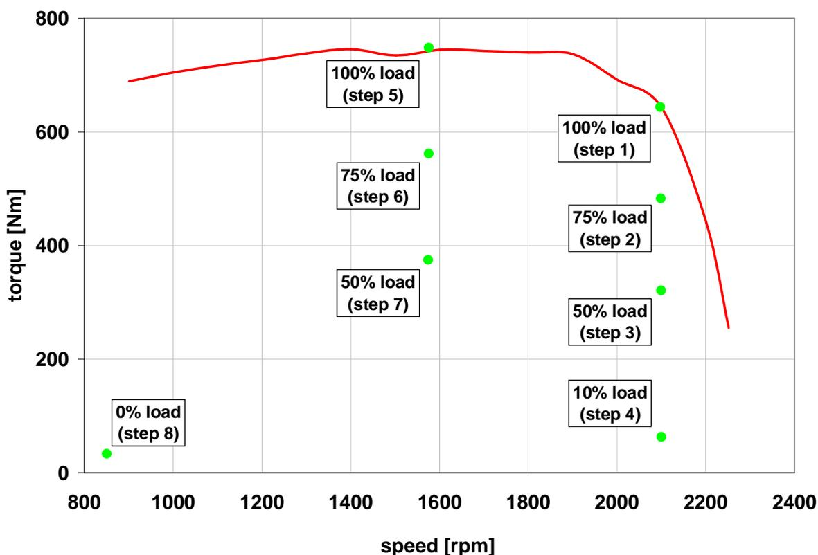
Figure 3 Applied stationary emission cycle based on NRSC
