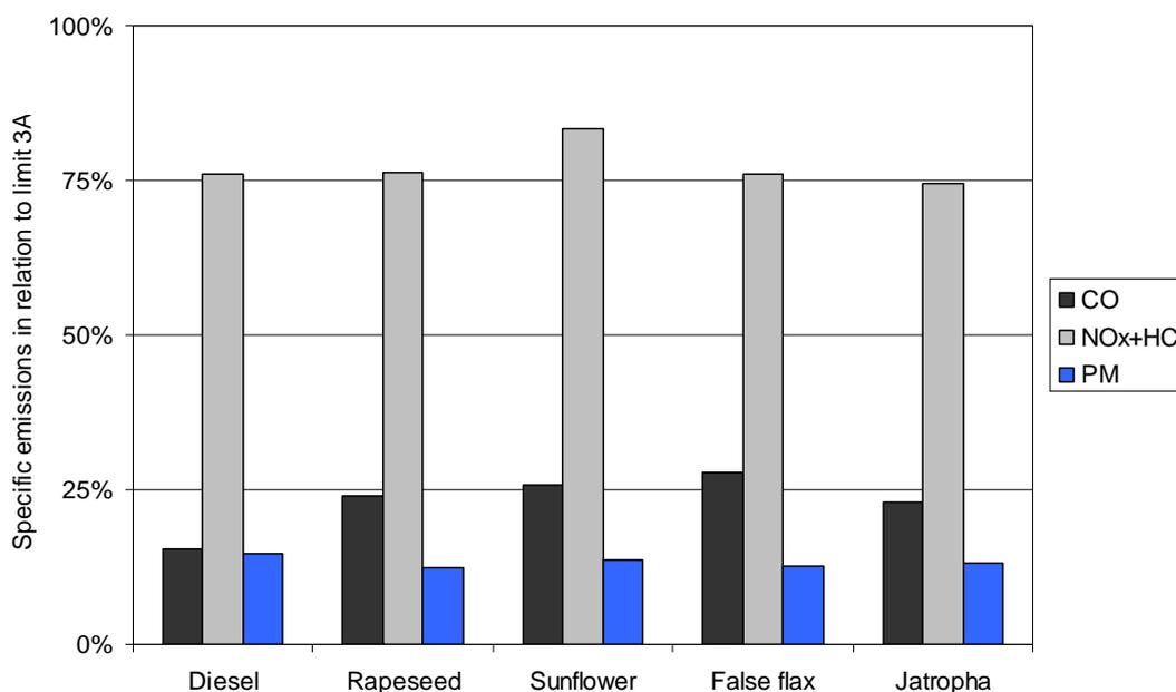
**Figure 9** Limited engine out emissions of stage 3A engine (ante DPF/DOC) with different fuels
