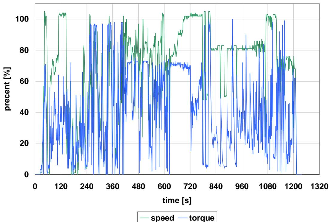
**Figure 4** Applied transient emission cycle based on NRTC
