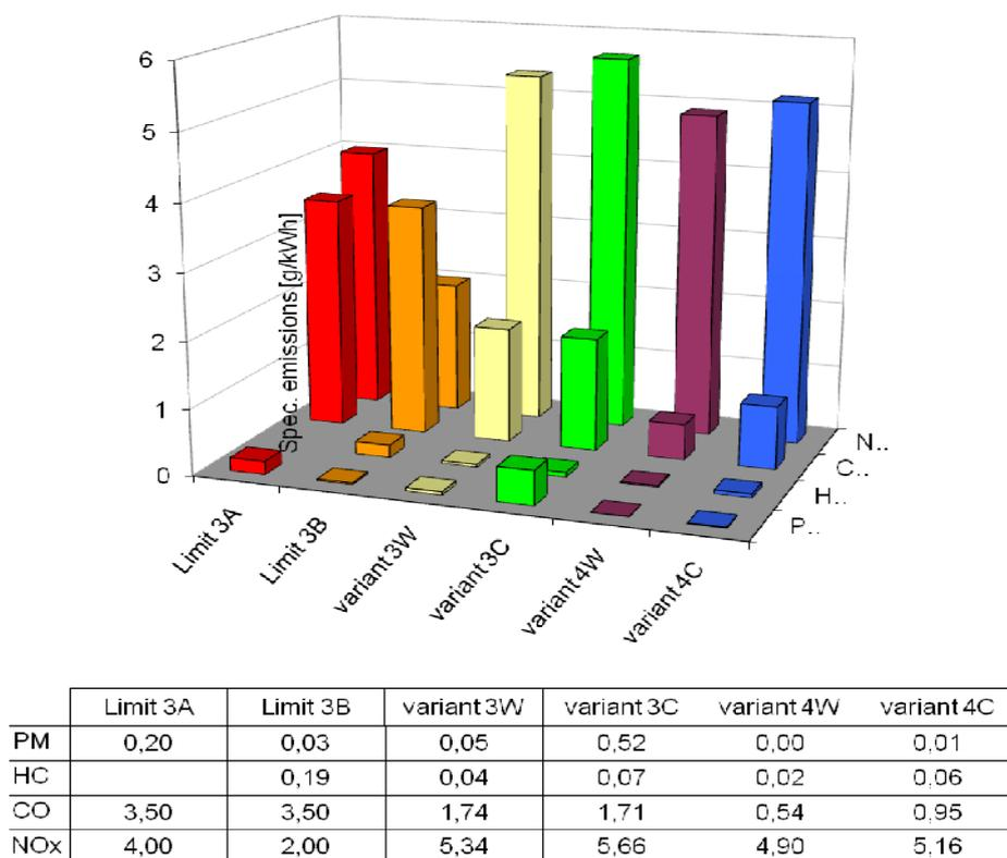
**Figure 8 Emissions of all evaluated engine/fuel configurations during the NRTC**
