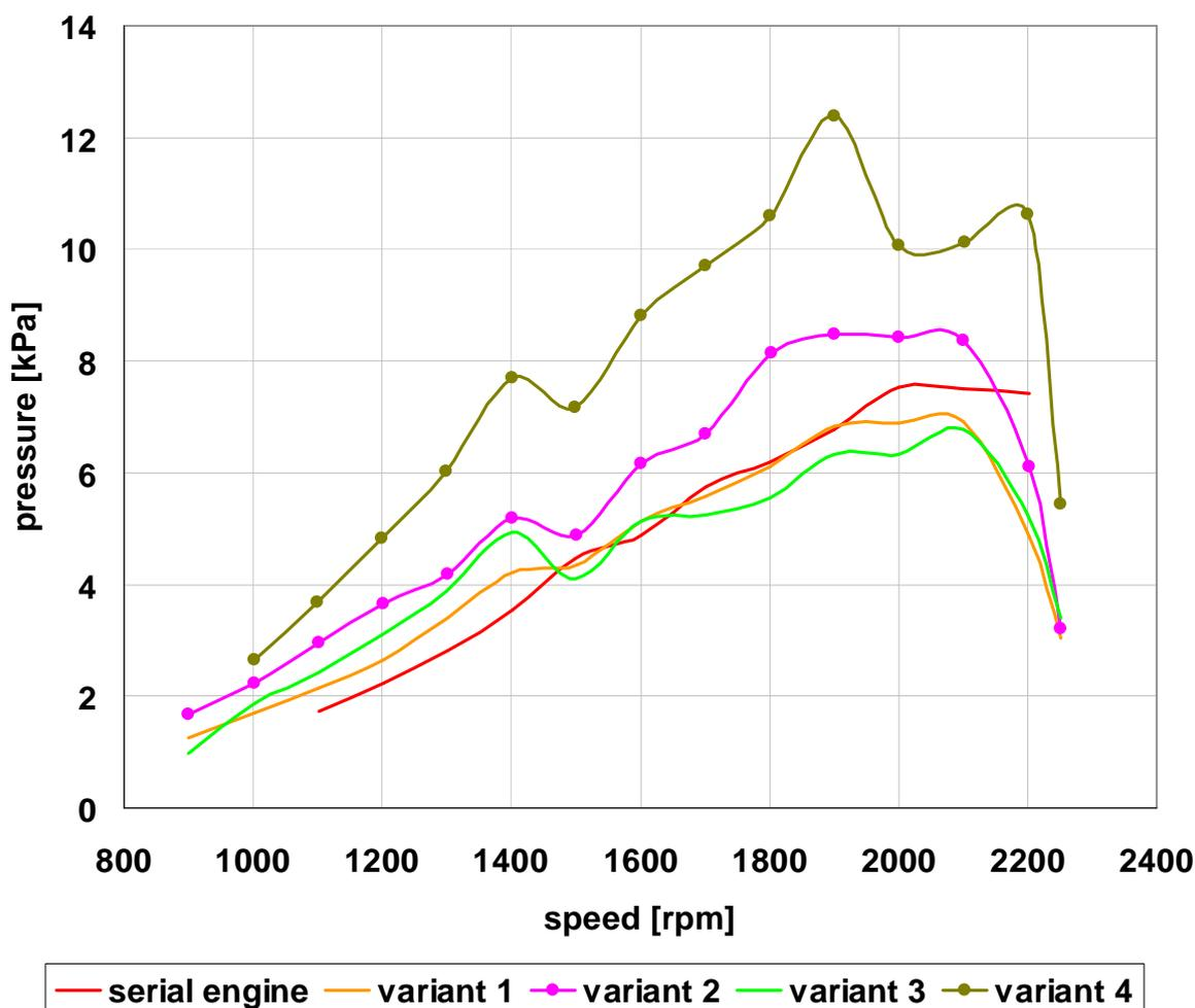
Figure 6 Exhaust gas back pressure of the four engine variants
