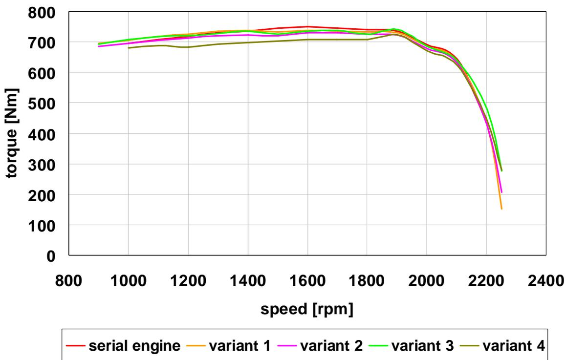
Figure 5: Torque curve of different engine configurations, diesel and rapeseed oil fuel
