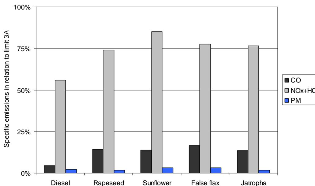
**Figure 10** Limited emissions of stage 3A engine (post DPF/DOC) with different fuels
