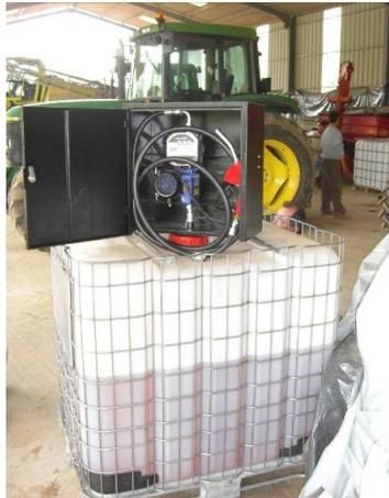
IBC with mounted filling station
