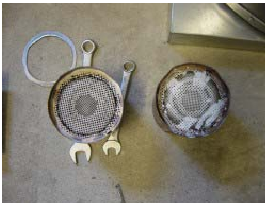
Figure 5: Charged and uncharged DPFs [12]
