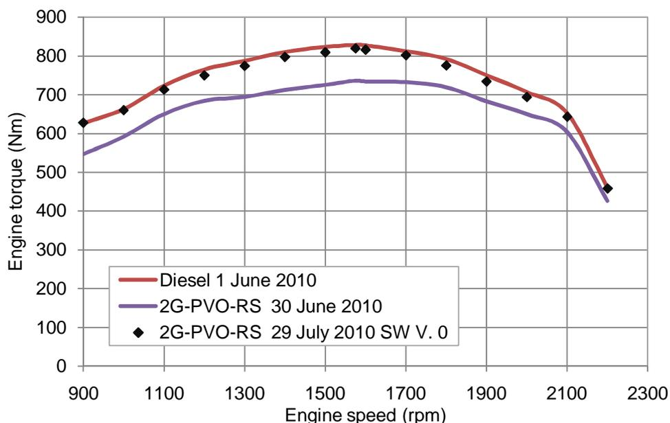
**Figure 6** Full load curves of the CD6068R000040 engine with diesel and rapeseed oil with series software and with rapeseed oil and modified software (vegetable oil SW version No 0)
