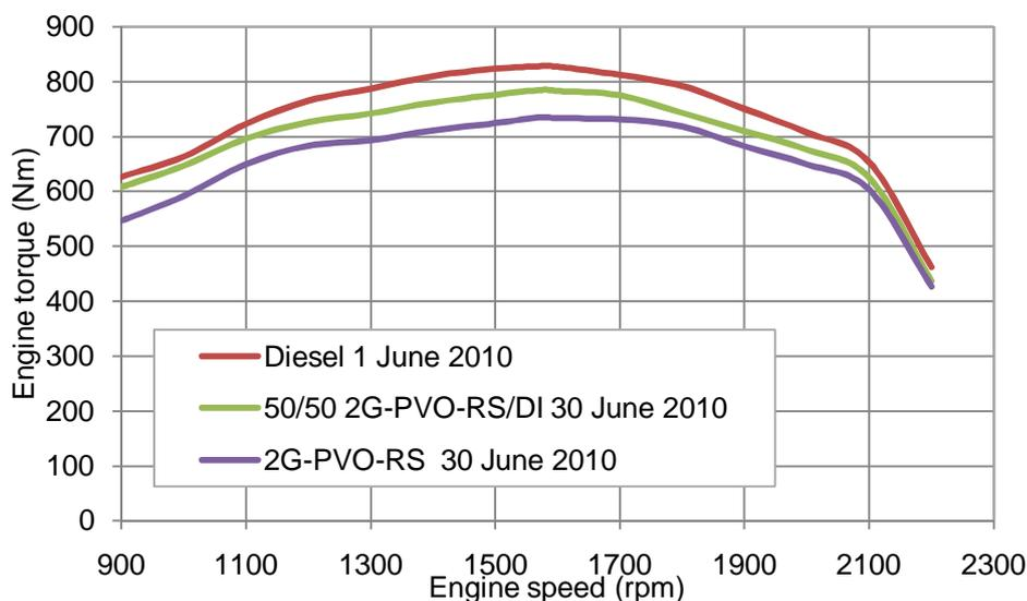
**Figure 5** Full load curves of the CD6068R000040 engine with diesel, 50% rapeseed oil in diesel and 100% rapeseed oil, series software
