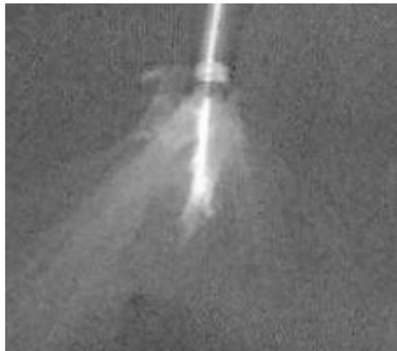
**Figure 3** RS injection on the nozzle test stand
