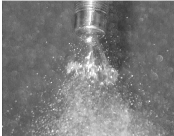
**Figure 2** DK injection on the nozzle test stand
