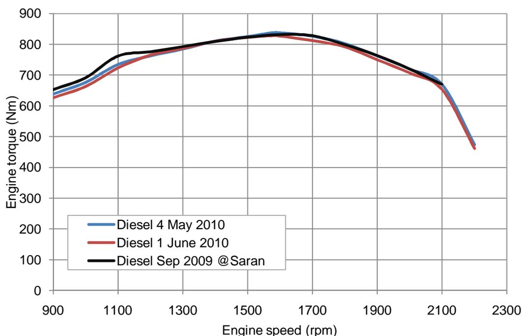
Figure 4 Reference full load curves with diesel fuel (engine CD6068R000040)
