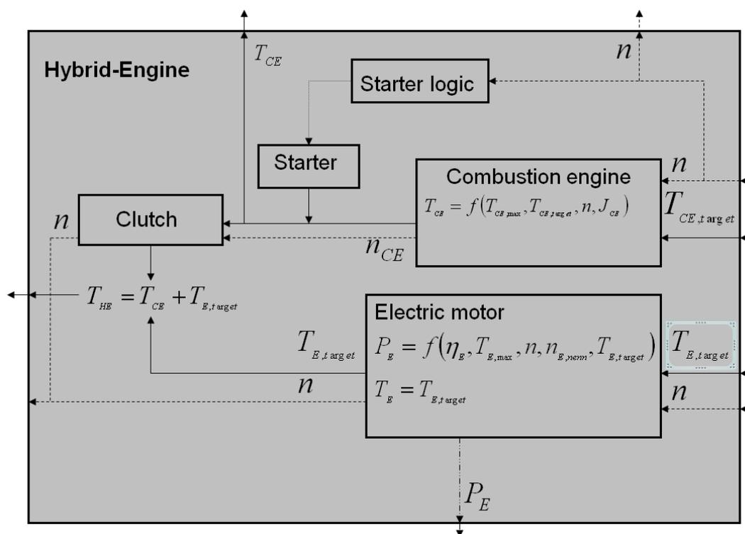
Fig. 11: diagram view model component: parallel driveline
