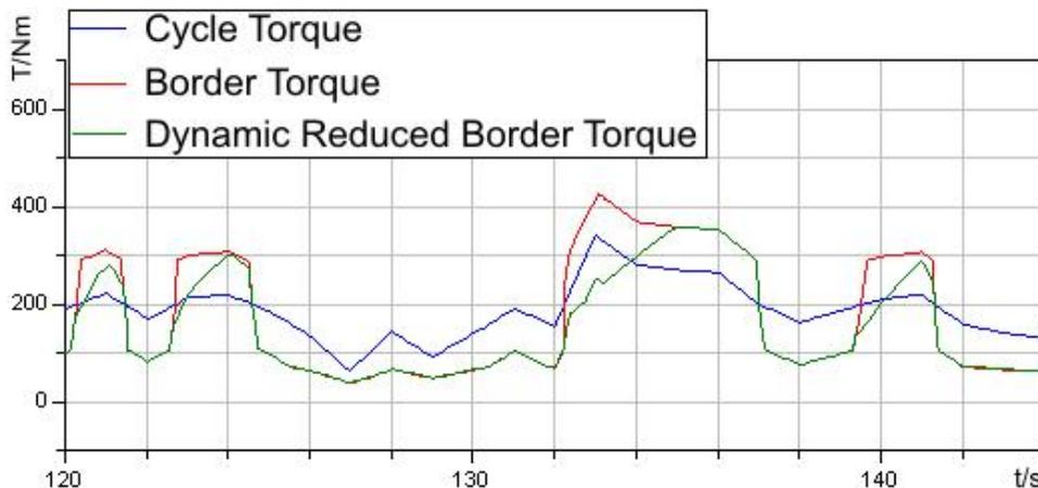
Fig. 23: Comparison of border-torque controller with/without additional dynamic reduction, torque curve of the simulation combustion engine
