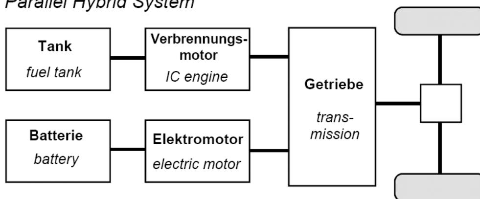
Fig. 2: Structure parallel hybrid system [2]
