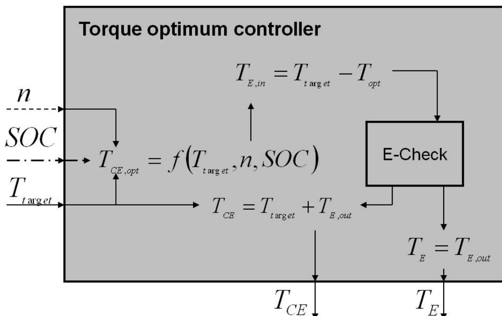
Fig. 18: optimum controller component
