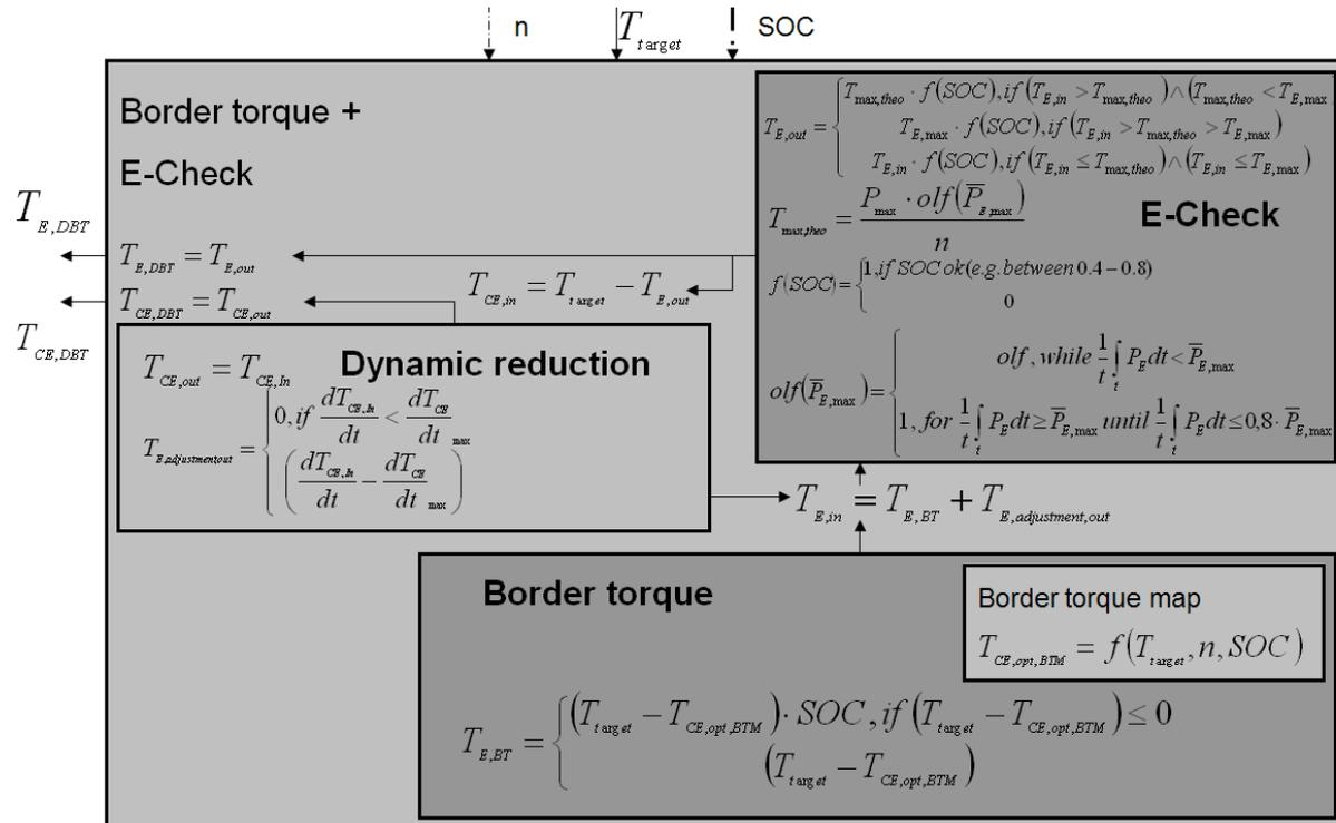
Fig. 22: Combination of border-torque and dynamic controller
