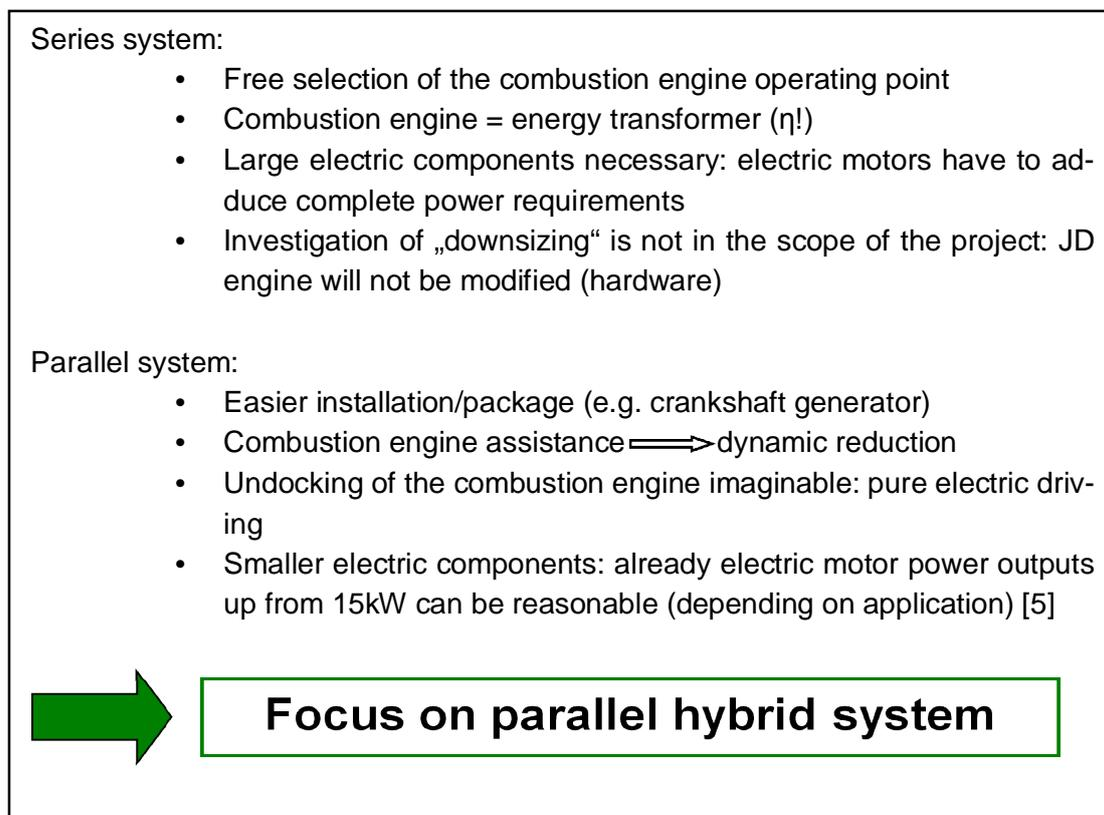
Fig. 6: Selection of the hybrid system structure
