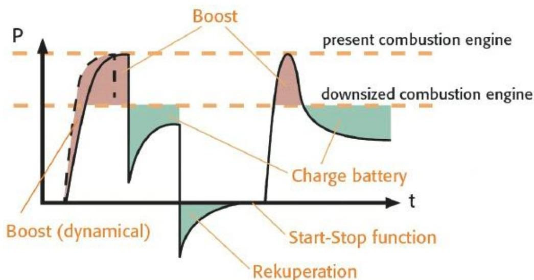
Fig. 3: Ideal operating profile for a hybrid application [4]
