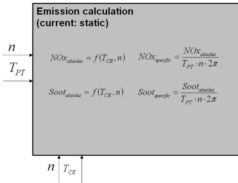
Fig. 14: Diagram view model component emission calculation
