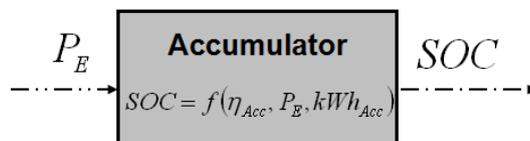
Fig. 10: accumulator model
