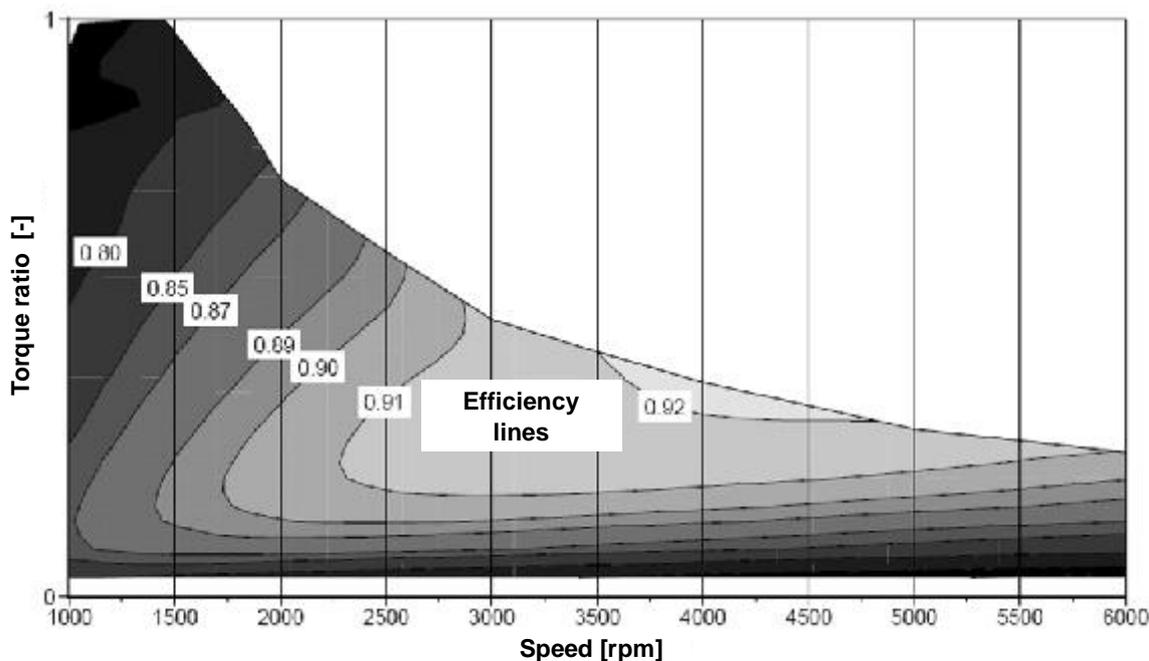
Fig. 8: Exemplary efficiency map of a synchronous machine [8]
