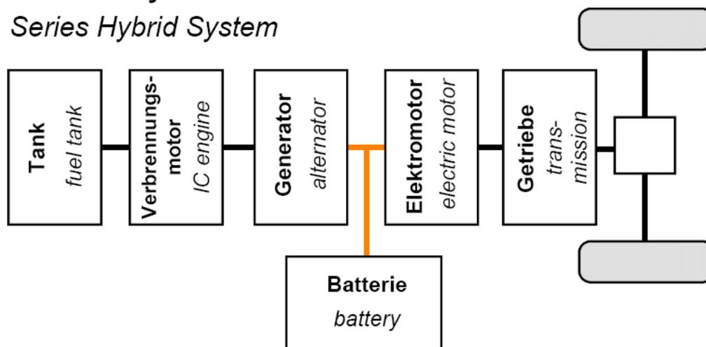
Fig. 1: Structure series hybrid system [2]
