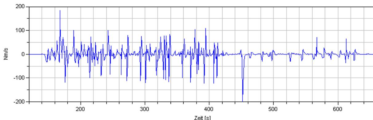
Fig. 19: Difference in torque gradients optimum controller / stand-alone combustion engine (cycle: NRTC)
