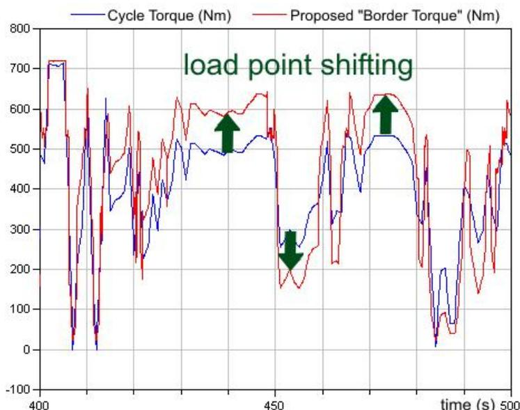
Fig. 20: Engine load shifting by border-torque controller
