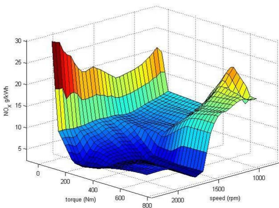
Fig. 16: measured specific NO<sub>x</sub> emission map (**stock application**) with rapeseed oil
