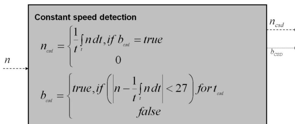
Fig. 24: Constant speed detection module
