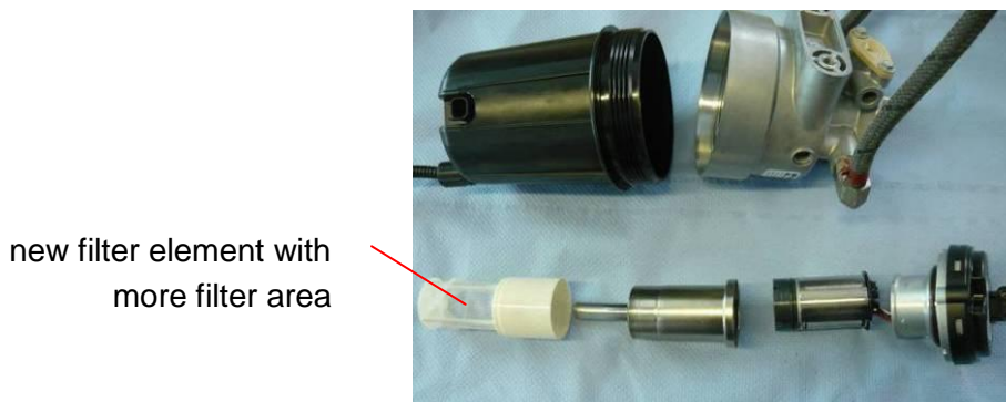
Figure 9: fuel pump with new components for 3B conversion, disassembled
