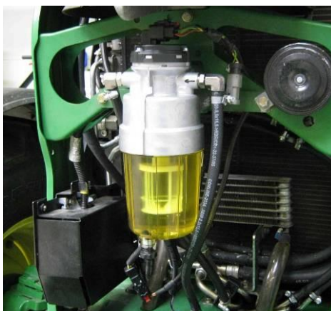
Figure 11: pre pressurization pump with pre fuel filter, mounted in front of the engine air cooler (concerted 3B tractor)
