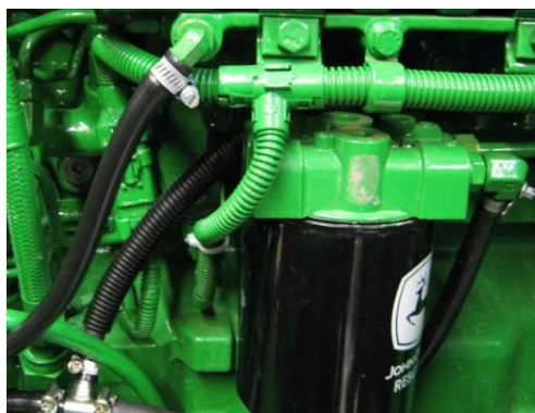
Figure 12: main fuel filter, mounted left side of the tractor
