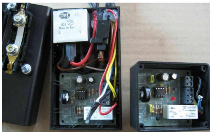
Figure 2: left side - prototype of new fuel preheating control unit, right side - old module only with preheating controller
