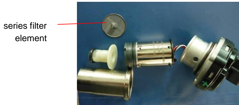
Figure 8: JD series fuel pump with small filter element, disassembled
