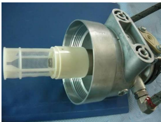
Figure 10: new filter connected to the fuel pump, assembled
